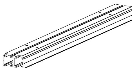
$$L_{\text{barra}} = L_{\text{vano}} + 100 + \left( \frac{L_{\text{vano}}}{n^{\circ} \text{ vetri}} \right)$$
